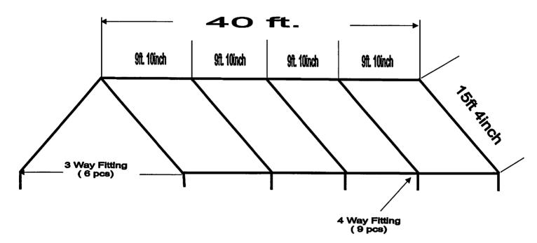
Step 2. Insert (B) 8ft Pipes to under 3Way and 4Way fitting at roof structure
