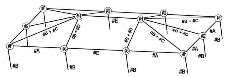
Step7. Install Bar Brace(12pcs) to any corner of inside frame.
